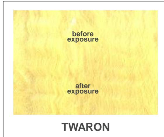
Due to its patented manufacturing process Twaron is showing less change of color after UV exposure. This visual perception builds confidence of inherent quality and performance characteristics.
