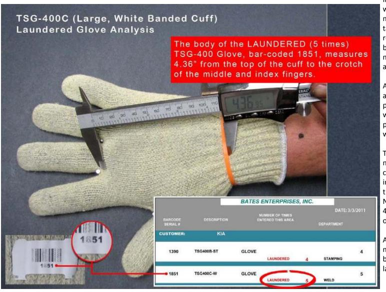
In this photo, the calipers were reset and measurements were taken against the reference point at the base of the crotch of middle and index fingers and the top of the cuff.
