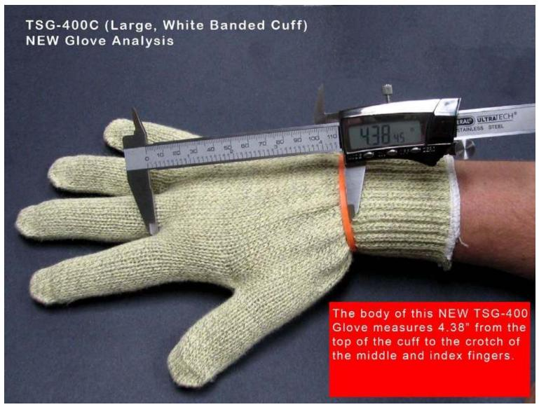
In this photo, the calipers were reset and measurements were taken for the body length of the glove.
