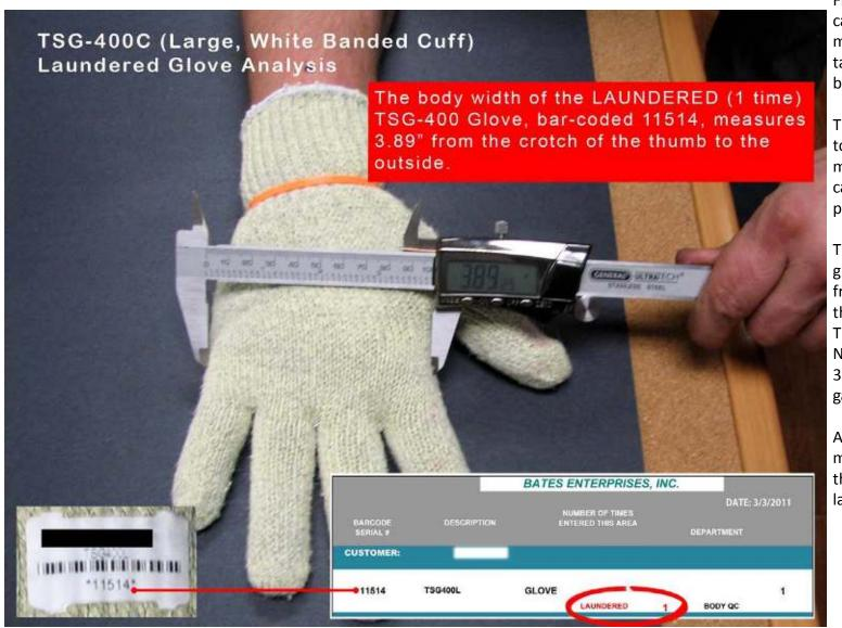
Finally, in this photo, the calipers were reset and measurements were taken for the width of the body of the glove.
