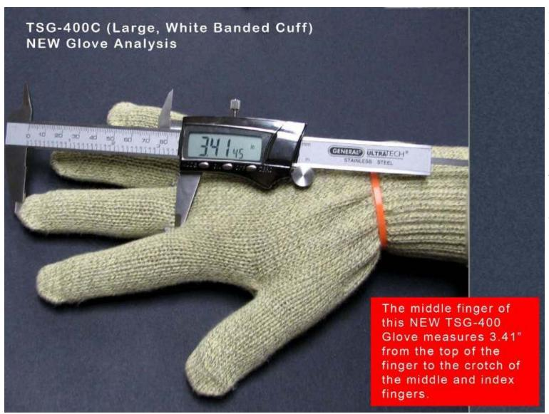
In this photo, the calipers were reset and measurements were taken for the middle finger length of the glove.
