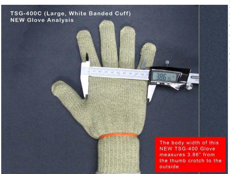
In this photo, the calipers were reset and measurements were taken for the body width of the glove.
