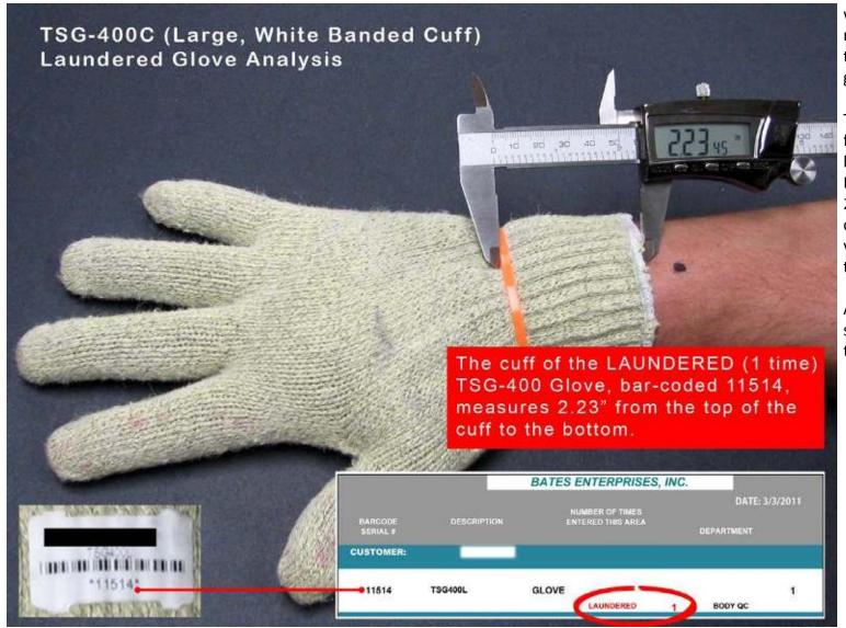
In this photo, the calipers were reset and measurements were taken for the cuff of the glove.
