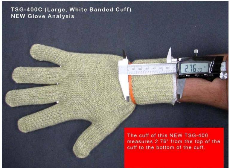
Contained herein is an analysis to dispel the assertion of major shrinkage between NEW gloves and Laundered gloves, model TSG-400C. Every attempt was made to be as accurate as possible. All the photos and information within are for internal use ONLY by Bates Enterprises, Inc.
