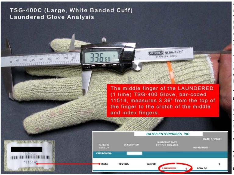
In this photo, the calipers were reset and measurements were taken against the reference points at the base of the crotch of the middle and index fingers and the top of the middle finger.
